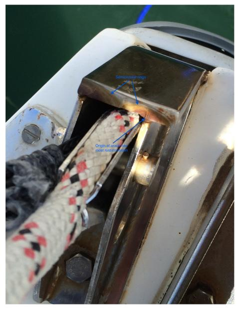
In my opinion the design of this plate lends itself to this type of failure because of the welding and difficulty in inspection. It is worth noting that Catalina Direct (with whom I have no commercial or other connection) offer a replacement that does not have the side plates, but a central lug instead.
