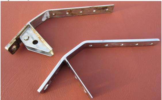
You can see that the gusset plates are welded in place to the main steel tang. Also the top (left) of the tang is doubled in thickness and I believe this is achieved by welding the second 'square' of metal onto the main tang, grinding smooth and then drilling the hole for the forestay attachment.
