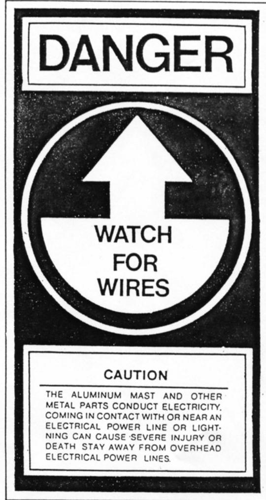
PART # WS2 ON FORWARD SIDE OF MAST 1'-0" FROM BOTTOM
